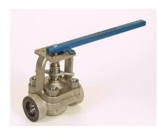
Conval Camseal® metal-seated ball valves provide zero body, seat, and stem seal leakage. The body/bonnet joint is not subject to pipeline stresses. There is no in-line body bolting to loosen and fatigue. Reliable, accurate ball alignment is achieved due to the robust engagement between the one-piece stem and the ball. The unique Camseal replacement cartridge design makes it possible to perform in-line servicing in 30 minutes. For F91 valves, no welding is required!
