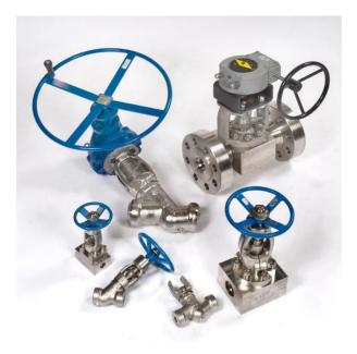
The valves shown were manufactured for one of our urea projects in the southwest. Urea applications are generally considered to be severe service, as a function of the pressures, temperatures and corrosive properties of the media. These gates, globes, checks and ball valves employed A182 F310MoLN (25-22-2) forgings with Ferralium 255 internals, and were delivered on-time. The forged materials were selected to comply with the Owner's requirements, and to provide long service life for the valves.
