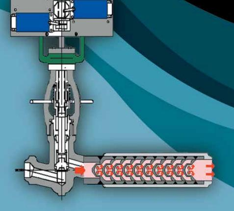
Conval Clampseal® Recirculation Bypass Valves are designed
